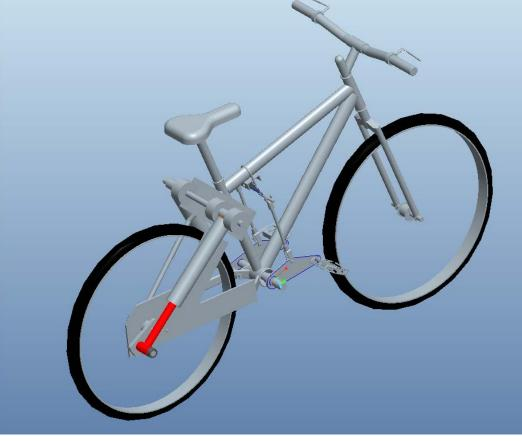
Other alternative designs were considered to design a cost effective hydraulic bicycle that could be mass produced. The design shown here consists of two cylinders and a unique pedaling system.
